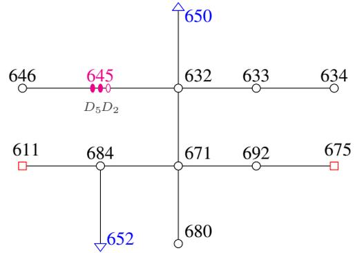
Figure 3. IEEE 13 node radial distribution test feeder
