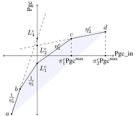
Figure 2. An illustrative example of a piecewise linear efficiency curve a set of linear functions defined by constraints (7a) through (7c) that apply efficiency curves to continuous as well as discrete resources at all nodes  $i \in N$ , time periods  $t \in T$  and slots  $k \in K_i$  for each linearization of piecewise function  $p \in \{1, \dots, P\}$ . In our models we have used  $P = 4$ .
