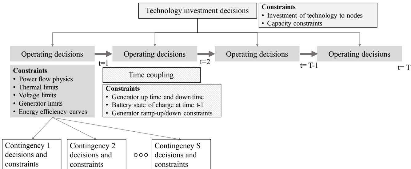
Figure 1. This flow chart describes the stages of the problem. At the top are the technology investment variables. The investments are applied at each operating time point (second level of the diagram). The operating decisions are connected via coupling constraints like ramping requirements. Each operating decision is further constrained by contingency requirements in the third stage (the figure only shows contingency constraints for  $t = 1$ ).
